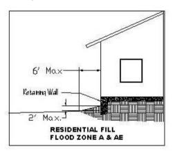
property ground, and limited to the area under the building envelope and shall extend no more than six feet (6') from any foundation or concrete slab (to achieve 3H:1V slope) as determined reasonable by the City Building Official or as approved in the subject Drainage Impact Study. The use of pier foundations for buildings located within the flood zone is highly encouraged by the City, as an alternative to filling of property located within the Flood Zone.
