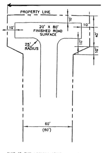
THIS IS THE MINIMUM REQUIRED. MORE MAY BE REQUIRED DEPENDING ON DRAINAGE, SEWERS, ETC.
